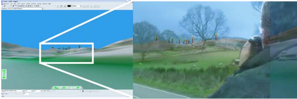
Figure 16 The view through the tree in Topos with OS map draped over the terrain. On the right, the semi-transparent photograph is overlaid over the relevant section of the same screenshot.
