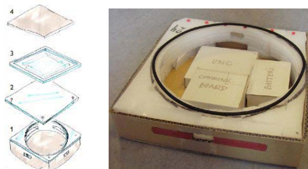
Figure 30. The tiles take form in the initial design sketches and mock-up produced by the Aarhus School of Architecture.
