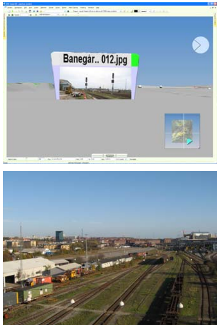
Figure 10 Pictures taken on-site, inserted automatically and oriented at the correct spot.
