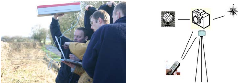
Figure 10 Site Tracker prototype and Site Tracker assembly expanded with remote control (mobile phone). Snapshot from a participatory field experiment
