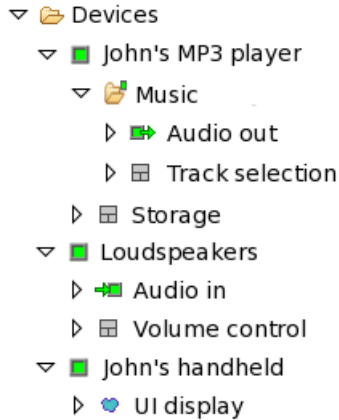
Figure 2.6: The tree of information about devices and services, as shown in John's PalCom browser in the music scenario.
