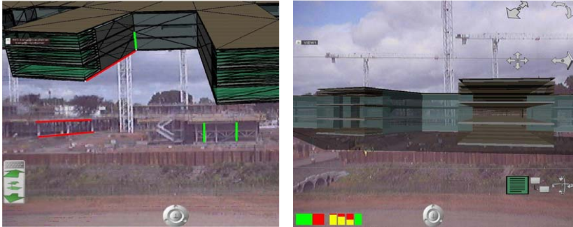
Figure 9: Overlaying live images with designed objects
