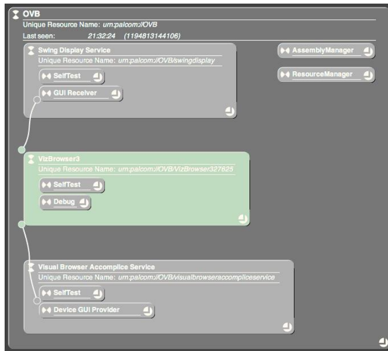
Figure 10: The topology of the Overview Browser device as shown by the OVBDevice itself. The device itself is depicted as the enclosing window encompassing five elements, three of which are the Swing Display Service, the Visual Browser Accomplice Service and an assembly reifying the viz3 assembly description, visualized as a kind of service and connected to the two services. Legend and visual detail descriptions can be found further down in the text.
